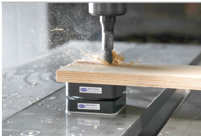
Innospann Cup and Mono-Base while clamping a wooden workpiece
